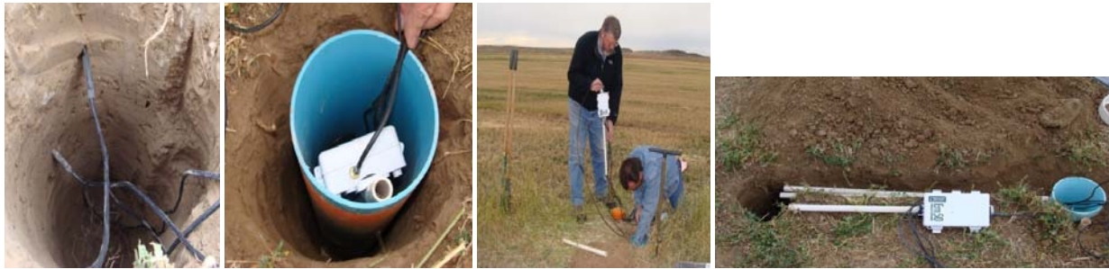
Figure 1. Echo soil moisture sensors inserted into the soil by depth, the meter, and installation.
